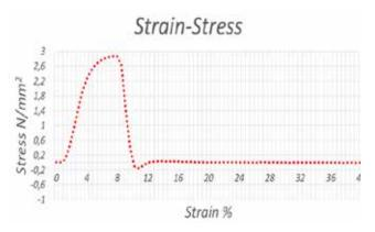
Figure. 3. Strain-Stress curve of multilayer membrane.
