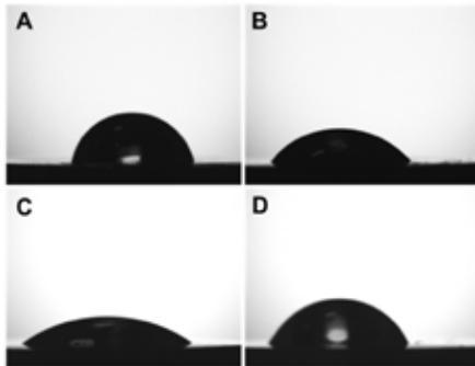
Figure 2. Measurement of water contact angle of non-CAP (A)Control (B)Group 1 (C)Group 2 (D) Group 3,  $83.73 \pm 2.23^\circ$ ,  $45.22 \pm 5.21^\circ$ ,  $30.21 \pm 2.34^\circ$  and  $76.12 \pm 1.21^\circ$ , respectively.
