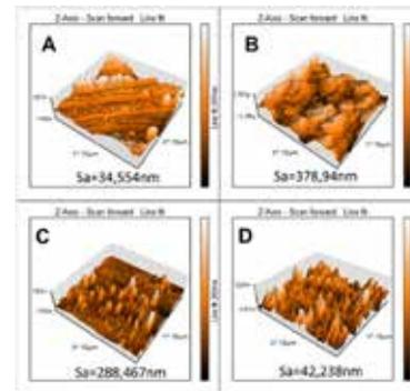
Figure 3. Representative 3D topographical view of titanium discs (A)Control (B)Group 1 (C)Group 2 (D) Group 3
